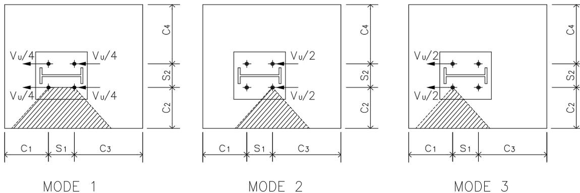
**Mode 1** Shear taken evenly by all anchor bolts, strength check against  $0.5 \times V_u$
