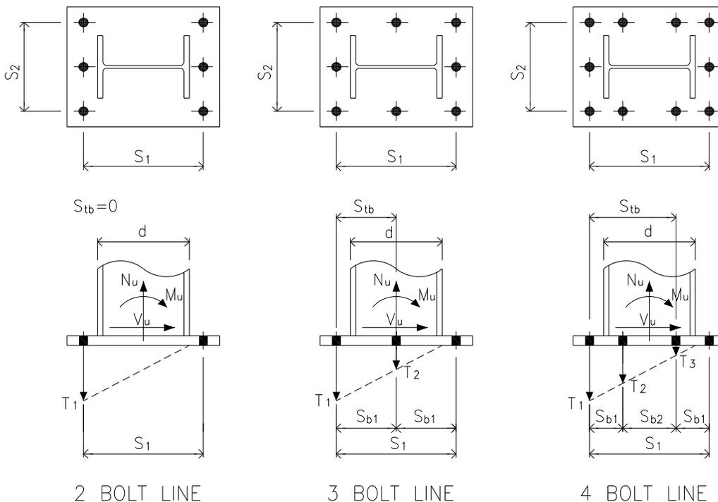
No of bolt line for resisting moment = 2 Bolt Line
