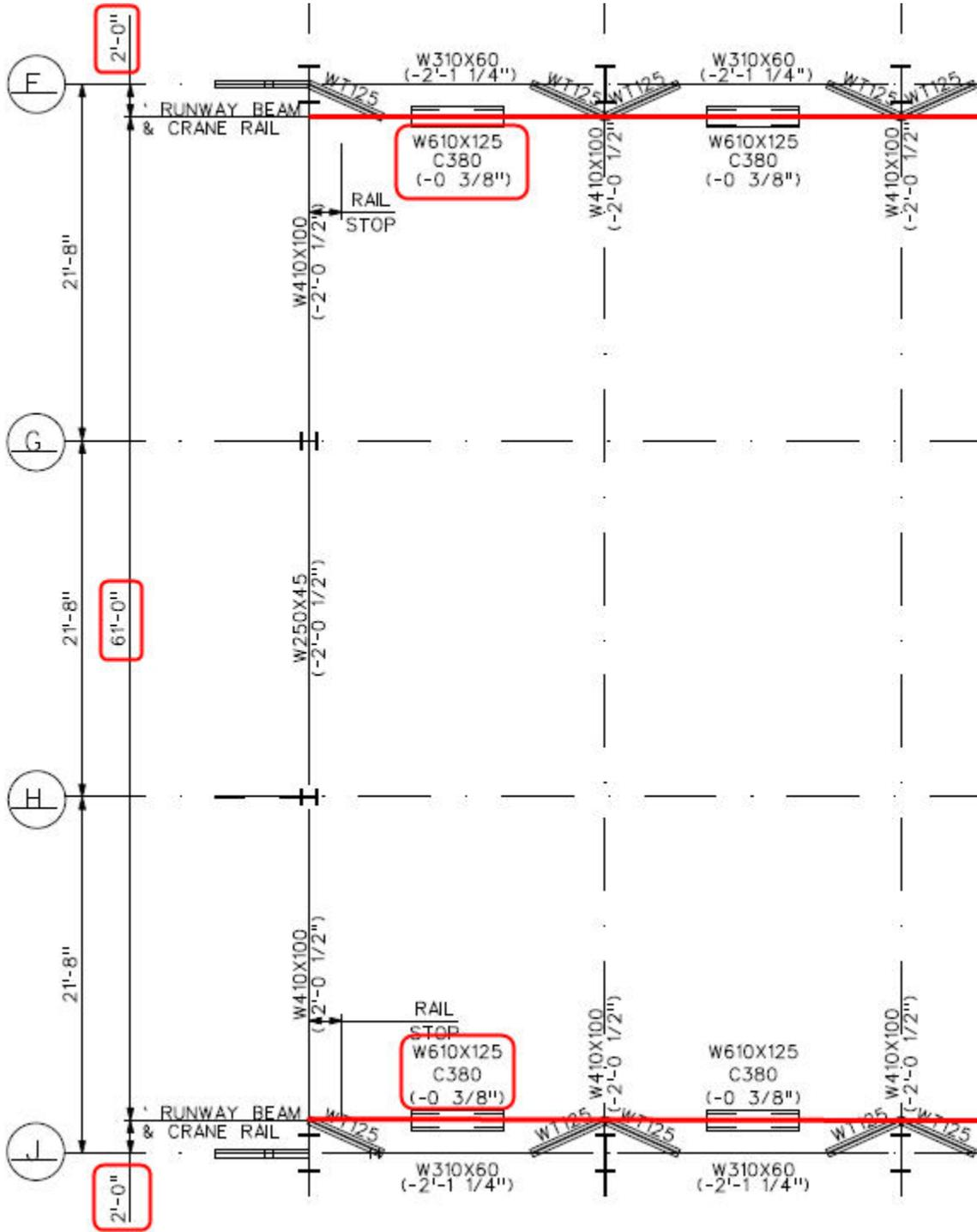
BRIDGE CRANE RUNWAY BEAM PLAN
