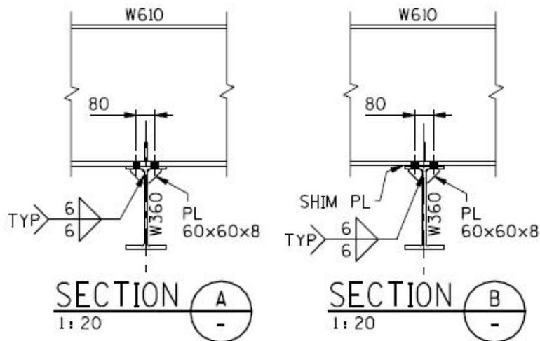
7.5 Tonne Underhung Crane W360x57 Runway Beam Support Point to Floor Beam Connection
